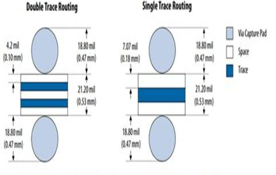
Escape Routing for Double and Single Traces for 1.00-mm Flip-Chip BGA
