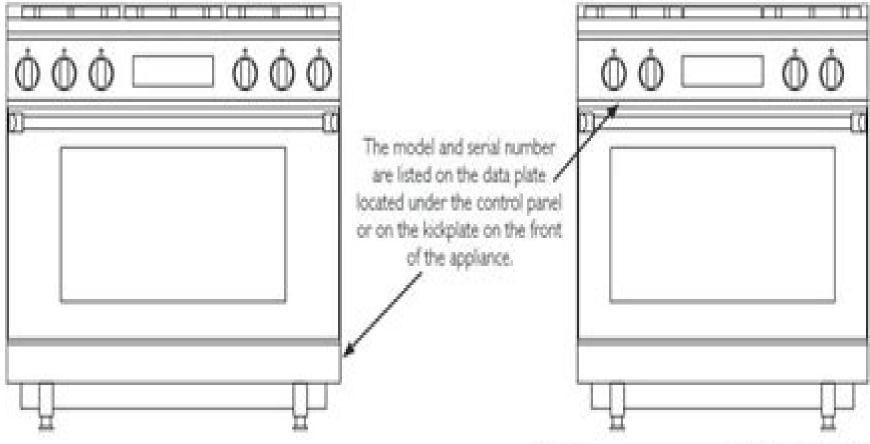
RATING PLATE - The location of the rating plate is shown above. The information on the rating plate defines the model, serial number, gas type (natural or liquid propane), operating pressures and burner BTU ratings. Keep this information for future reference. It is essential for proper identification of the unit when requesting additional information or factory support.
