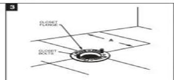
INSTALL CLOSET BOLTS Install closet botts in flange channel, turn 90°, and slideimo place 8° (152 mm) apart and parallel to wall.
